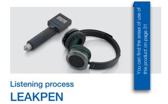
The LEAKPEN is the smallest and simplest leak detector. It is an aid to the drinking water supplier, just as a voltage tester is an aid to an electrician. During prelocation of leaks, the LEAKPEN can be used to measure the structure-borne sound and is often used in connection with water meter readings or for hydrant and slide gate valve inspections.
